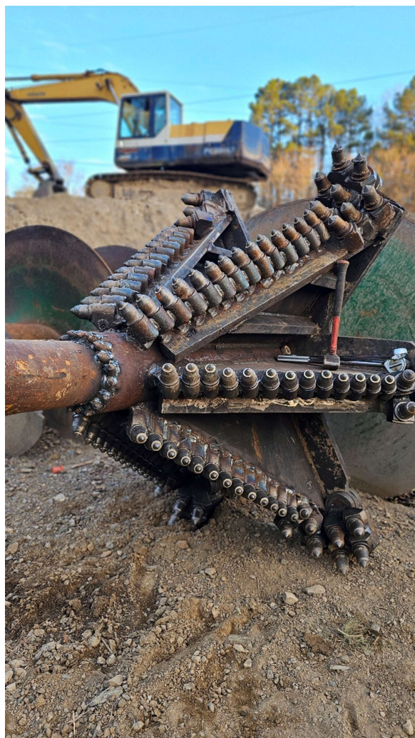
Cutting head for 60" pipe bore under Malvern Highway
